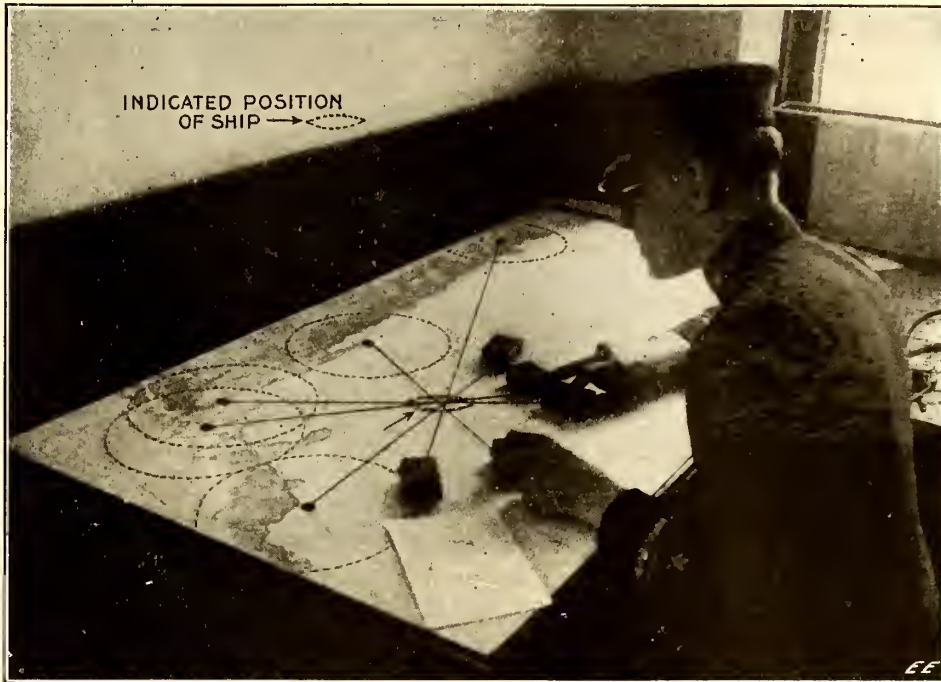
Sandy Hook Got Captain Wood's Appeal at a Distance of Sixty Miles. Mantoloking Was Even Further Away. These Stations and Also That at Fire Island, by Their Land Lines Into New York, Reported the Bearings of the Lancastrian From Their Respective Positions. The Central Station, Within Ten Minutes Then Sent All Three Bearings by Radio to the Leland Line Ship and Her Master's Mind Was at Ease.
