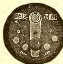
Detectagraph Rheostat, especially made for amplifying circuits.
