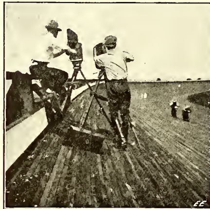
Taking a "Slow Movie" of a Motorcycle Race at 200 Pictures Per Second.
