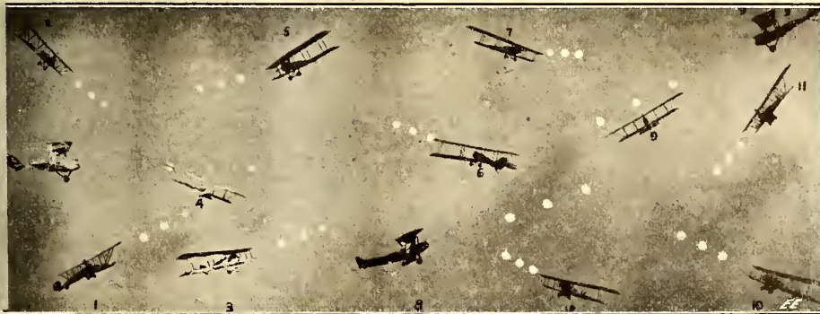
Clever Electric Chart Board for Instructing Aviators in Firing at Enemy Planes. After the Dummy Machine Gun Has Been Sighted, the Lights Are Flashed On and the Gun Is Checked With Them.
